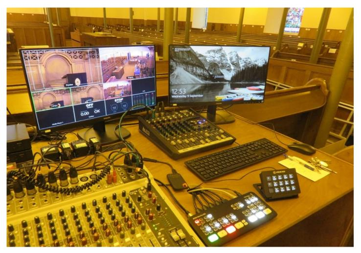
This does look pretty complicated but for the purposes of controlling the cameras we can ignore the two larger control panels with little knobs and sliders – these are both related to the sound system.
