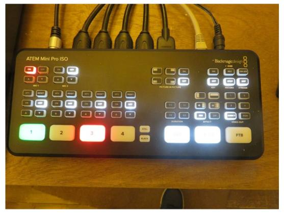
This allows the operator to switch between cameras, set up the "next" camera, broadcast to YouTube and loads of other stuff which we are unlikely to use, at least in the beginning.
