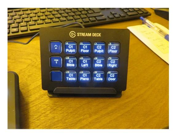
Each of the PTZ cameras has 6 pre-set positions and each position has a dedicated button. There is no requirement for the operator to manually swing a camera round or to adjust focus – that is all taken care of by the prepared position. Selecting a button automatically moves the camera to the perfect position.
